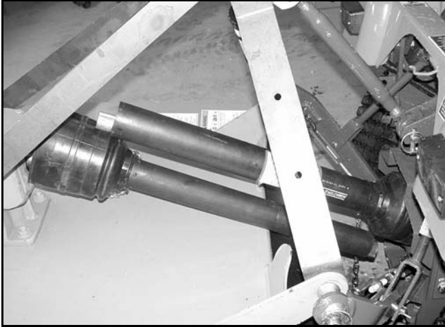
Figure 2. Drive Halves Placed Parallel
